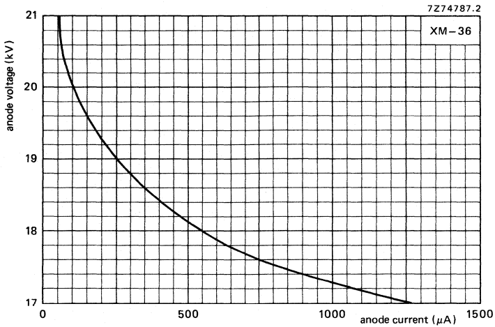
Fig. 2 0,5 mR/h isoexposure-rate limit curve, according to JEDEC 94, measured according to TEPAC103A.
